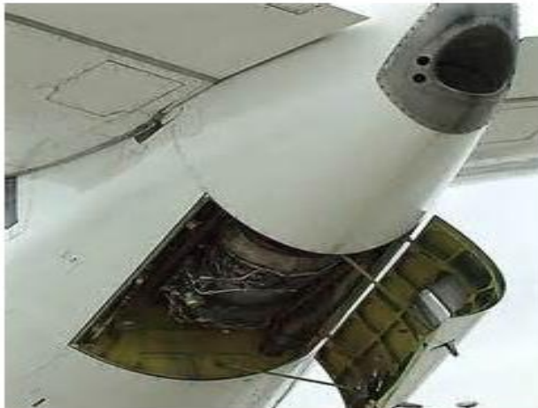
Auxiliary Power Unit inside the aircraft
