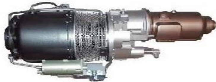
Auxiliary Power Unit outside the aircraft
